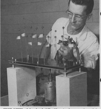
HIGH LEVEL of free-hand skill with a touch-up gun is needed by painters in Section 4221-2 to apply carbon coating .040 of an inch thick. Bruce Higgins sprays 16 glass balls on "gear train."
